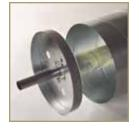
12" diameter drums allow for lower headroom requirements. An enclosed barrel houses the dead axle assembly and protects the factory lubricated springs from direct contact with environmental elements. The inherent strength provided by the spiral barrel minimizes axle deflection providing smoother operation. Because the curtain is attached by screws and not seamed to the barrel, replacement of either independent assembly is cost-effective, quick and easy.
