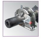
A cam-action spring tension holding device allows guick, easy and equal adjustment of the tension on all springs simultaneously from one end of the door. The cam tensioner bites into the axle helping to eliminate the unwanted spinning of the axle during the initial spring loading or adjustment process.
