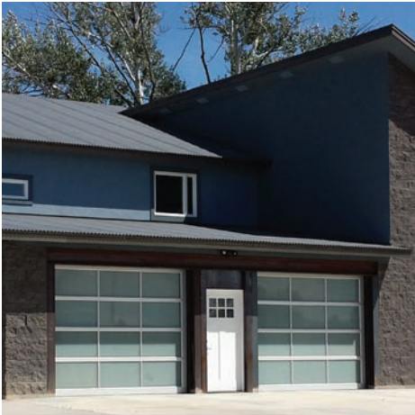
Narrow Profile, ArmorBrite white rails with 1/8" tempered black glass
